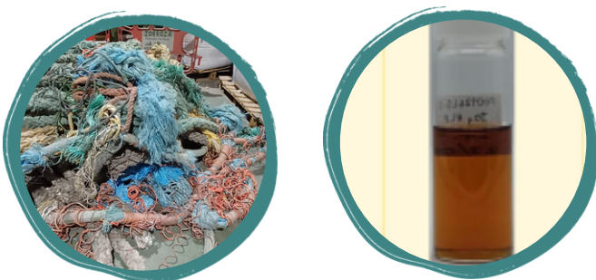
Above Left: EOL gears at port. Above Right: an example of the TACOIL ® produced from pyrolysis in laboratory trials.
