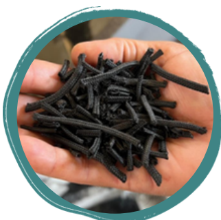
LEFT: Cut segments of the PA tuna purse seine net. RIGHT: Monofilament spools produced from recycled polyamide. Images courtesy of Saretu
